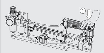
Disconnect the air before proceeding with the adjustment.
