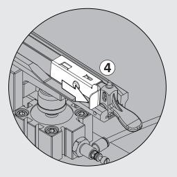
3 - Open the slider closing trigger.
